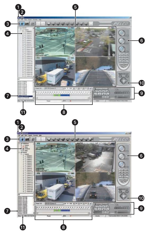
Figure 17. DX8100 Client Application Main Window
